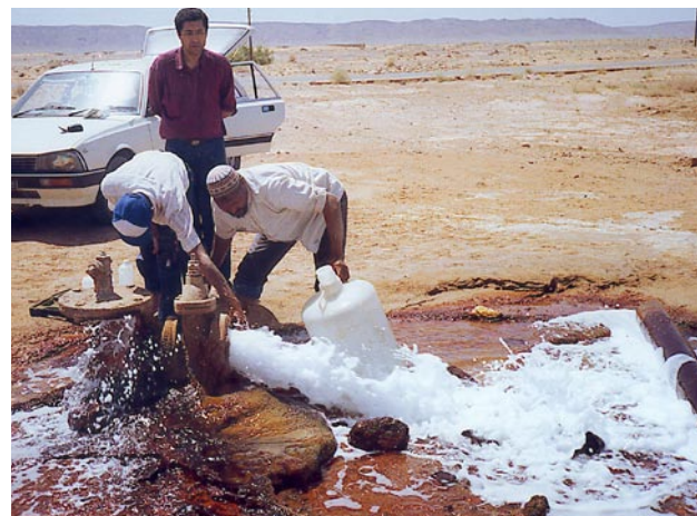
Collecting water samples for isotope measurements from an artesian well in Morocco. Photo: IAEA
